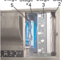
This Ventless Hood consists of a Five stage Air Purification System.
